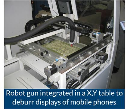
Robot gun integrated in a X,Y table to deburr displays of mobile phones
