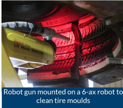
Robot gun mounted on a 6-ax robot to clean tire moulds
