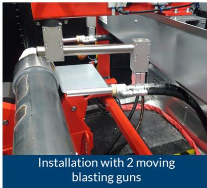
Installation with 2 moving blasting guns
